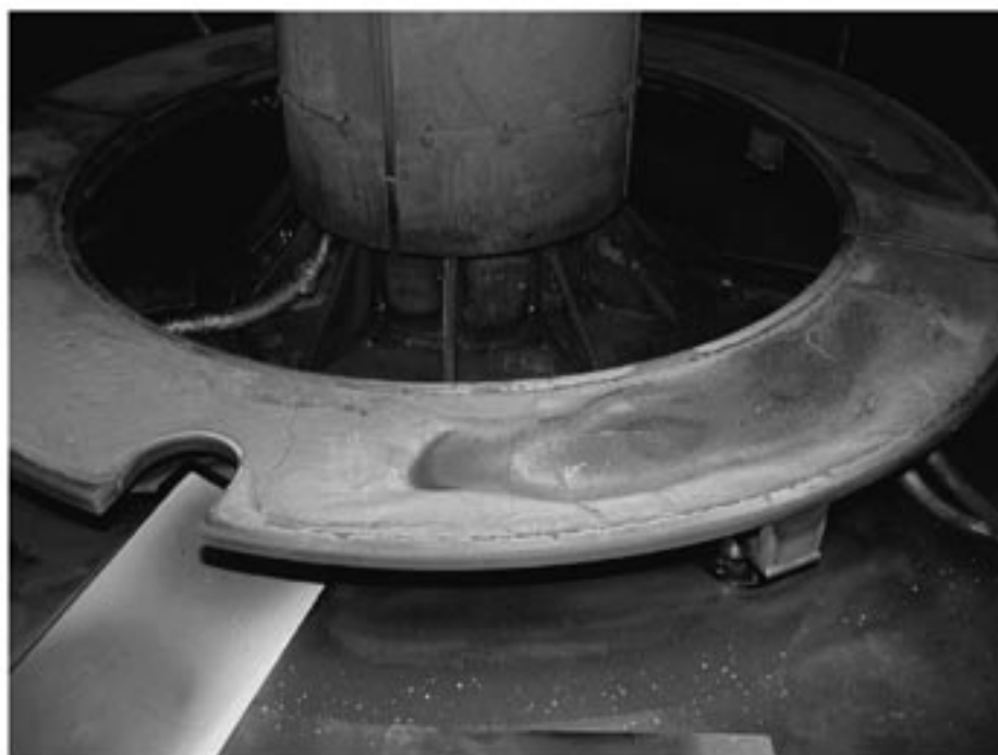
Fig. 11. Photograph of the interior of CDX-U immediately following venting after the second lithium tray campaign. The central columnar structure is the center stack, with heat shields. The tray encircles the center stack, and at this point is filled with oxidized lithium. The notch visible in the left foreground permits an on-axis interferometer chord. The floor is the lower vessel heat shield.
