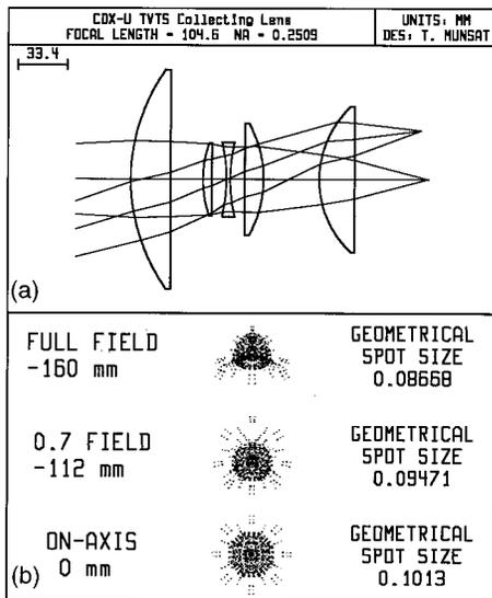
FIG. 3. (a) Five-element collection lens, with center and edge image-focus shown. All elements are stock catalog items. (b) Ray-trace spot-size analysis. Spot size is  $\leq 0.1$  mm over the full field of view.
