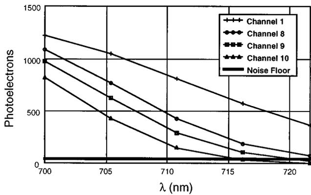
FIG. 6. Modeled spectra for four selected spatial channels. Shown are channels 1 (center), 8, 9, and 10 (near edge). Channels 11 and 12 (edge, not shown) have fewer than three spectral points above the noise floor.
