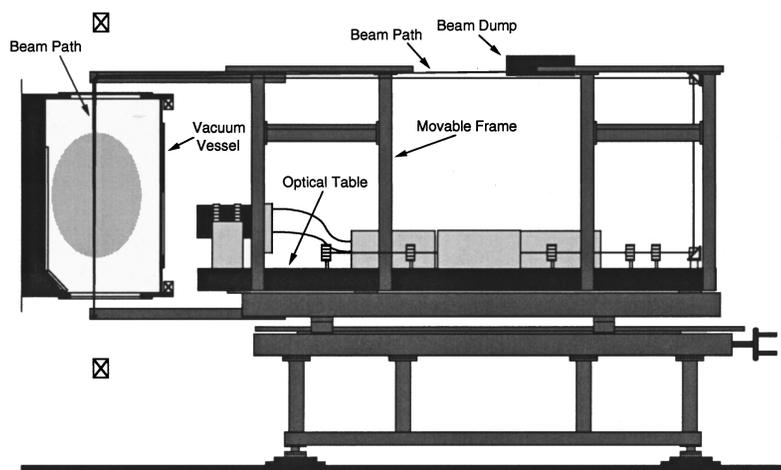
FIG. 1. CDX-U TVTS system with half cross section of vacuum vessel. Visible are two-pass vertical beam path, beam dump, and optical table housing laser and all collection optics.
