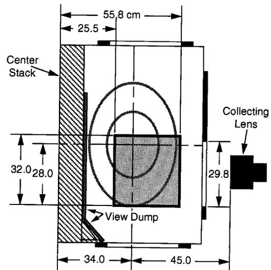
FIG. 2. Close-up of vacuum vessel cross section with TVTS coverage indicated. One elongated plasma radius is imaged, and the entire system is scannable over nearly 70% of the major-radial plasma extent.
