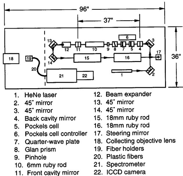
FIG. 5. Optical table layout. All laser components, collection optics, spectrometer, and camera fit onto a 3 ft  $\times$  8 ft optical table.
