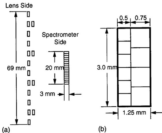
FIG. 4. (a) Fiber-bundle tips, with rearrangement between the lens-image side and at the spectrometer entrance slit shown. Gaps between bundles at the lens side allow for full beamline coverage while still fitting channels into the spectrometer entrance slit. (b) Close-up of a single fiber bundle. Custom dimensions are attainable with stock (0.5 and 0.75 mm) square-fiber sizes.
