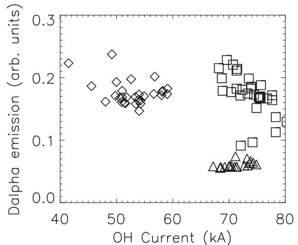
FIG. 2.  $D_\alpha$  emission at peak plasma current for discharges without lithium wall coatings (diamonds), with modest levels of lithium wall deposition (6–10 Å/min, squares) and with extensive lithium wall coatings produced by evaporation from the lithium tray limiter (triangles).
