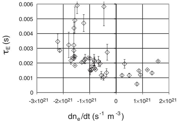
FIG. 5. Measured energy confinement time versus the density pump-out rate ( $dn_e/dt$ ). The density pump-out rate is a good measure of the degree to which recycling is suppressed.
