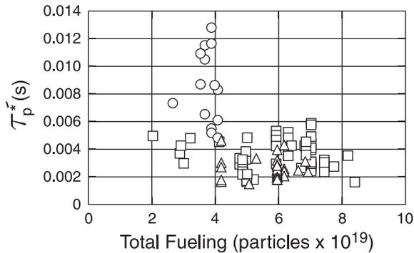
FIG. 3. Effective particle confinement time  $\tau_p^*$  versus total number of deuterons injected for discharges with varying levels of lithium wall conditioning. The triangles denote results with the full lithium tray liquefied (2000 cm<sup>2</sup>), squares denote electron beam evaporation and a 600 cm<sup>2</sup> liquid lithium area, and circles denote operation with passivated lithium (no active evaporation or heating).
