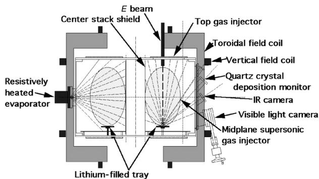
FIG. 1. Schematic of CDX-U, with the lithium and fueling systems, and the electron beam injector.
