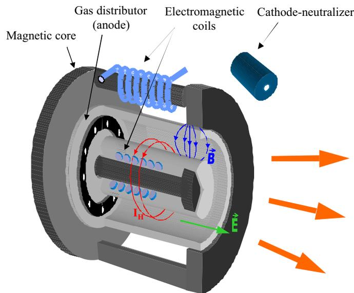
Plasma thrusters for current space applications employ xenon propellant. Xenon is relatively easy to ionize and store onboard the spacecraft. It also has a high atomic number (54), which means a lot of mass per ionization energy expended. The ionization energy is an unavoidable inefficiency; in the range of exhaust velocities most useful for current space applications – about 15 km/sec – this energy loss for once-ionized xenon is less than 10 percent of the exhaust
